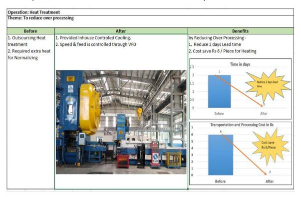
Provided in-house control cooling conveyor online after forging process this gives benefits of cost saving Rs 6 (Rs 5/Piece for heat treatment and Rs 1 for Transportation) and reduced lead time by 2 days as shown in figure No:5
